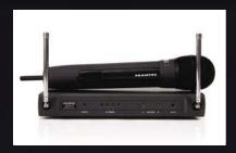
Multi-function receiver, 4 switchable frequencies and the latest PLL quartz tuning technology. Licence free in the UK on channel 70. Features include LEDs on receiver showing Power On, AF Peak level, RF Level and Diversity Channel A or B, and variable gain jack plug output. This handheld version is fitted with a high quality dynamic capsule with battery life in excess of eight hours.
