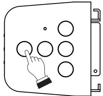
**Step 3.** After ensuring that the USB connection indicator is lit blue, release the Power switch. Initialization is complete, causing the unit to start.
